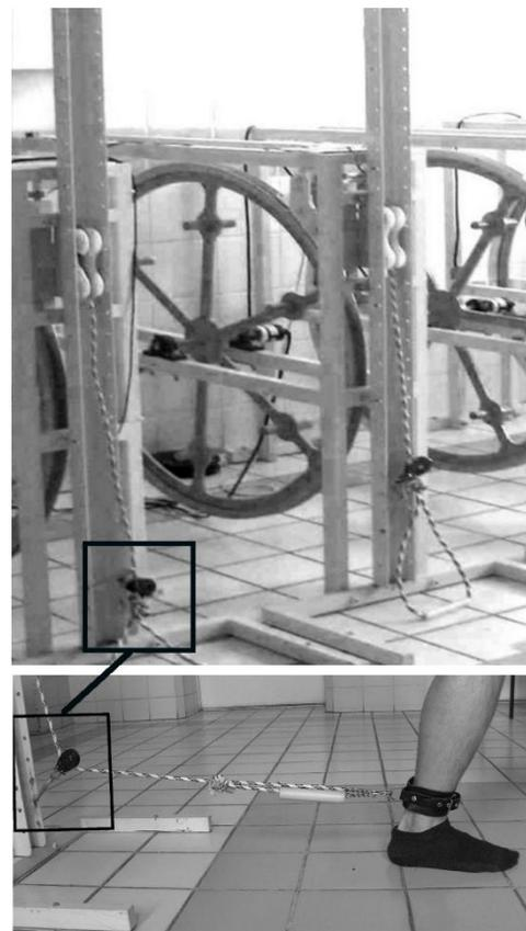
**Figure 1.** The Inertial Training and Measurement System (ITMS) and a way of mounting the rope to the ankle.
