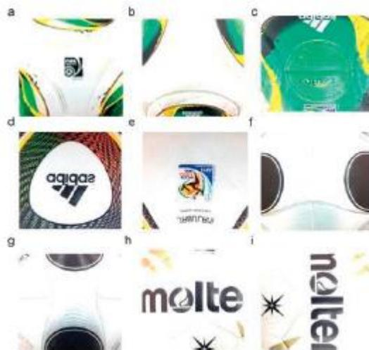
**Fig. 8.** The soccer balls used in the test panel orientations of respective soccer balls. (a,b,c) Adidas Cafusa: small grip texture with 32 modified panels; (d,e) Adidas Jabulani: small ridges or protrusions with 8 panels; (f,g) Adidas Teamgeist II: small protuberances with 14 panels; (h,i) Molten Vantaggio (conventional ball): smooth surface with
