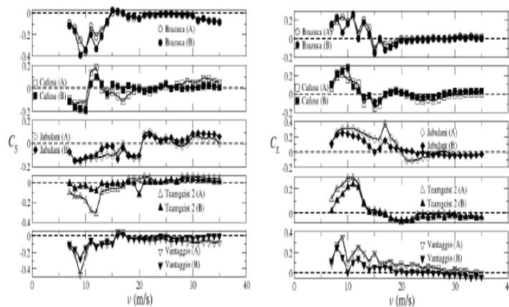
**Fig.17.** Speed-dependent side (left) and lift (right) coefficients for each of the two orientations of the five balls tested. Horizontal dashed lines show where  $C_S$  and  $C_L$  change sign (Goff et al., 2016).
