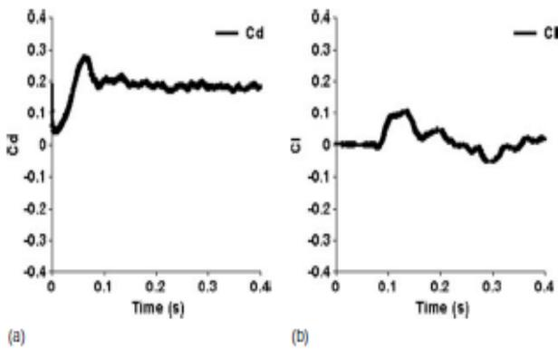
**Fig.14.** Drag coefficient vs time (a) and lift coefficient vs time (b) on CFD (Asai et al., 2007).
