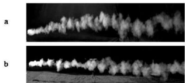
**Fig.16.** Comparison of the vortex street of a knuckleball (a) with that of a normal straight ball (b). A large scale undulation is evident in the knuckleball (Hong et al., 2010).
