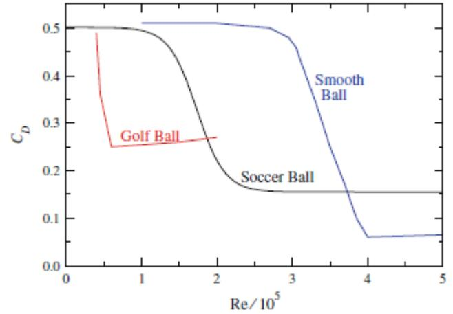
**Fig. 2.**  $C_D$  as a function of  $Re$  for a smooth sphere, a soccer ball and a golf ball (Goff, 2013).
