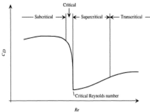
**Fig. 1.** Flow regimes on a sphere (Mehta & Pallis, 2001).
