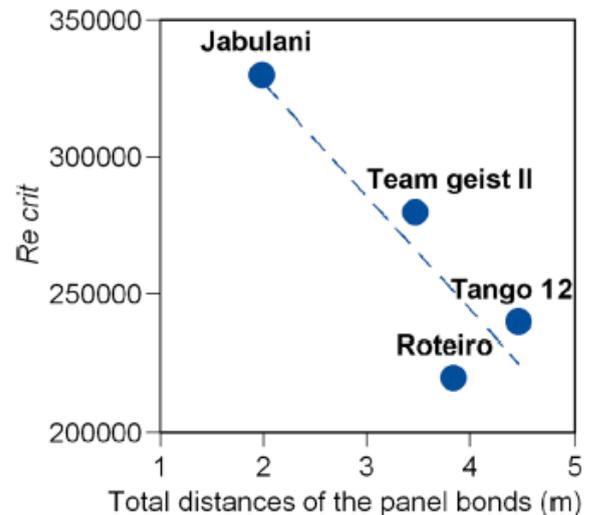
**Fig. 6.** Correlation between the extended total distances of the panel bonds and the critical Reynolds number (Asai & Seo, 2013).
