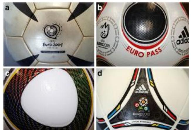
**Fig. 7.** Photographs of soccer balls. (a) Adidas Roteiro with 32 pentagonal and hexagonal panels. (b) Adidas TeamgeistII : small protuberance with 14 panels. (c) Adidas Jabulani: small ridges with 8 panels. (d) Adidas Tango 12: small grip texture with 32 modified panels (Asai & Seo, 2013).
