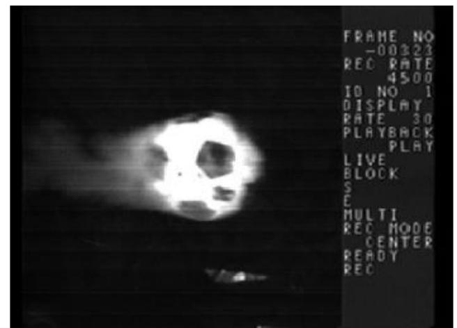
**Fig. 4.** Visualization of the flow around the ball after a high-velocity kick (29m/s).the boundary layer separation point receded to ~120 from the front stagnation point (Asai et al., 2007).
