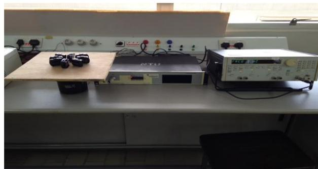
**Figure 1: Set up for the pedometer shake test using a mechanical shaker**
